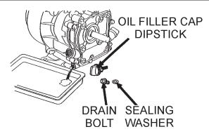
Figure 16. Engine Oil Plug
